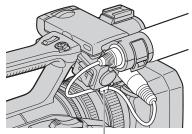
Hook the cable in the outer cable holder.
