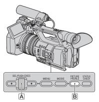
You can customize the picture quality by adjusting picture profile items such as [GAMMA] and [DETAIL].
