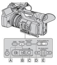
You can adjust and fix the white balance according to the lighting conditions of recording environment.
