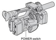
**1** Slide the POWER switch to ON while you press the green button.
