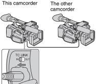
The time code of this camcorder synchronizes with that of the connected camcorder. [TC IN] appears on this camcorder screen.
