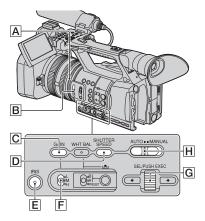
You can adjust the image brightness by adjusting the iris, gain or shutter speed, or by reducing the light volume with the ND filter  $\square$ .
